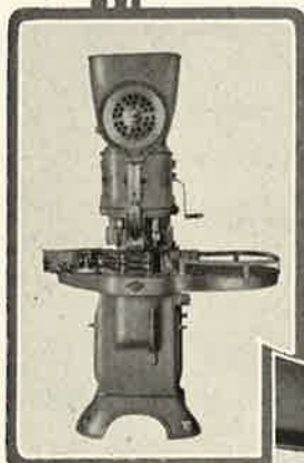
One of three "Liquid" Rotary Crowners with which the plant is equipped.
